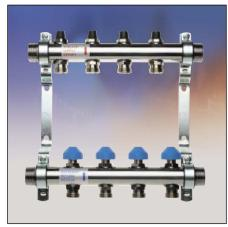
Brass round pipe manifolds in the sizes  $1\frac{1}{2}$ " and 2". Ball valve shutoff, regulating valve or flowmeter are screwed to the manifold pipe. Available in modular design (2/3/4/6 outlets) or from 2-20 outlets.
